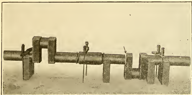
FIG. 28.—Two-Throw Crankshaft—Fracture Cut Away for Welding.
